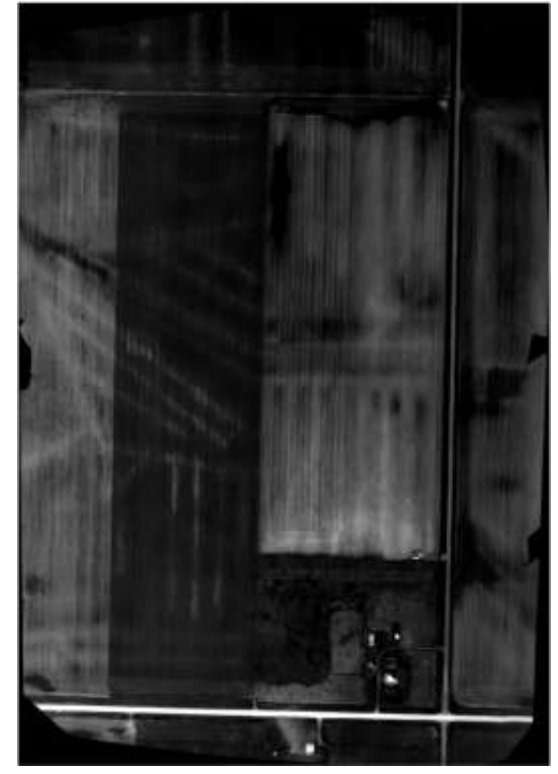
Field Thermal Infrared Orthomosaic from One Day After 3'' Rainfall Showing Drainage Pipe Patterns. (Compare to As-Built Drainage Map.)
