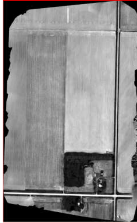
Field Thermal Infrared Orthomosaic from One Day Before 3'' Rainfall Exhibiting no Drainage Pipe Responses.
